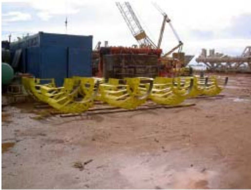
Flange protection cages
